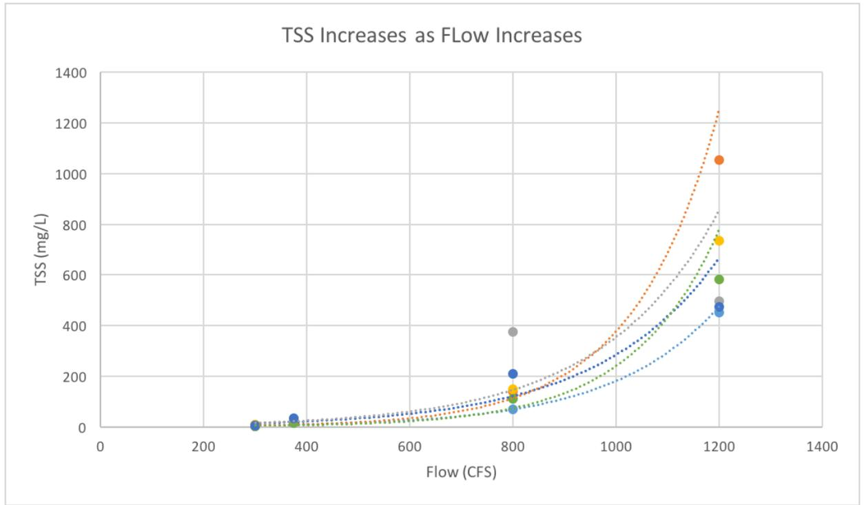
Figure 5. This graph plots all TSS data based on TSS (mg/L) and the flow (ft/s<sup>3</sup>) of the Catawba River during sampling.
