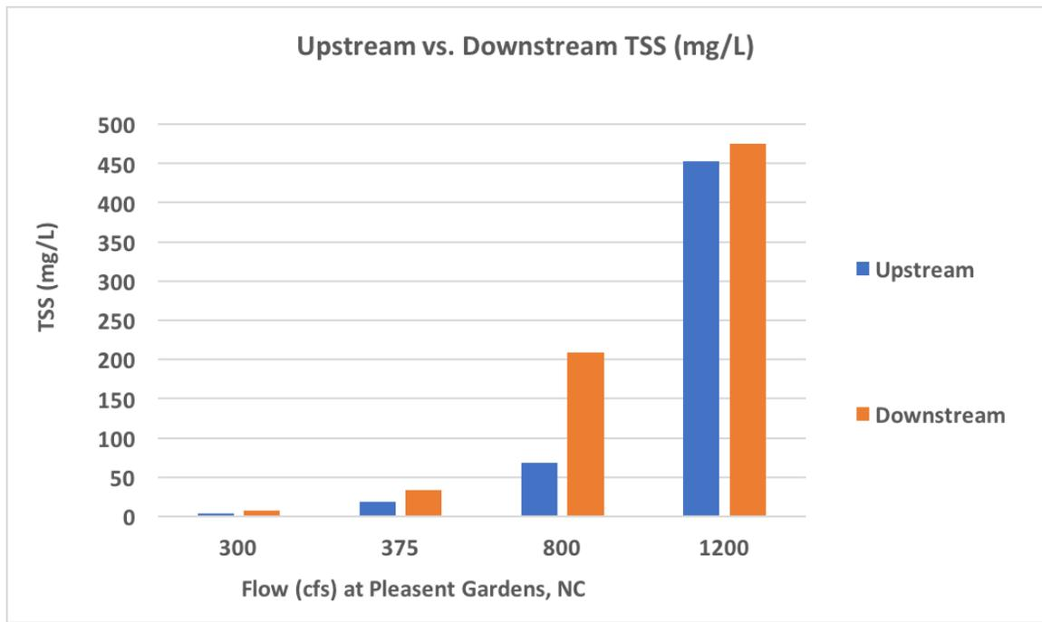
Figure 6. This graph plots the furthest upstream and downstream samples based on TSS (mg/L) and the flow (ft/s<sup>3</sup>) of the Catawba River during sampling.
